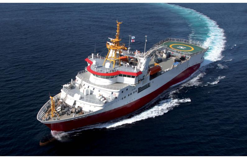
The vessels are the first of a new generation high efficiency 12/14 streamers Seismic research vessel where safety, efficiency, redundancy and high transit speed have been emphasised. The vessels will be fitted with comfortable accommodations for 60 persons, supporting the latest standards and regulations. The powerful propulsion plant will give the vessels excellent towing capabilities and higher transit speed than similar vessels within the seismic segment.
